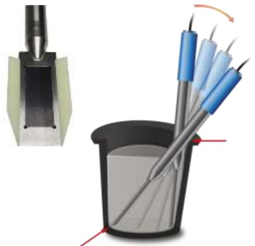
**Please consider:** Concretes which do not comply with standards can tend to bleed. Such concretes are difficult to measure with SONO-WZ but also with kiln drying test. In such cases it can come to measurement deviations.
