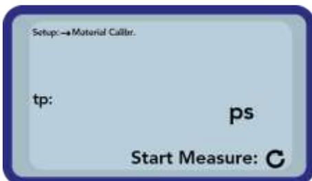
To start the measurement push the button „Measurement“
