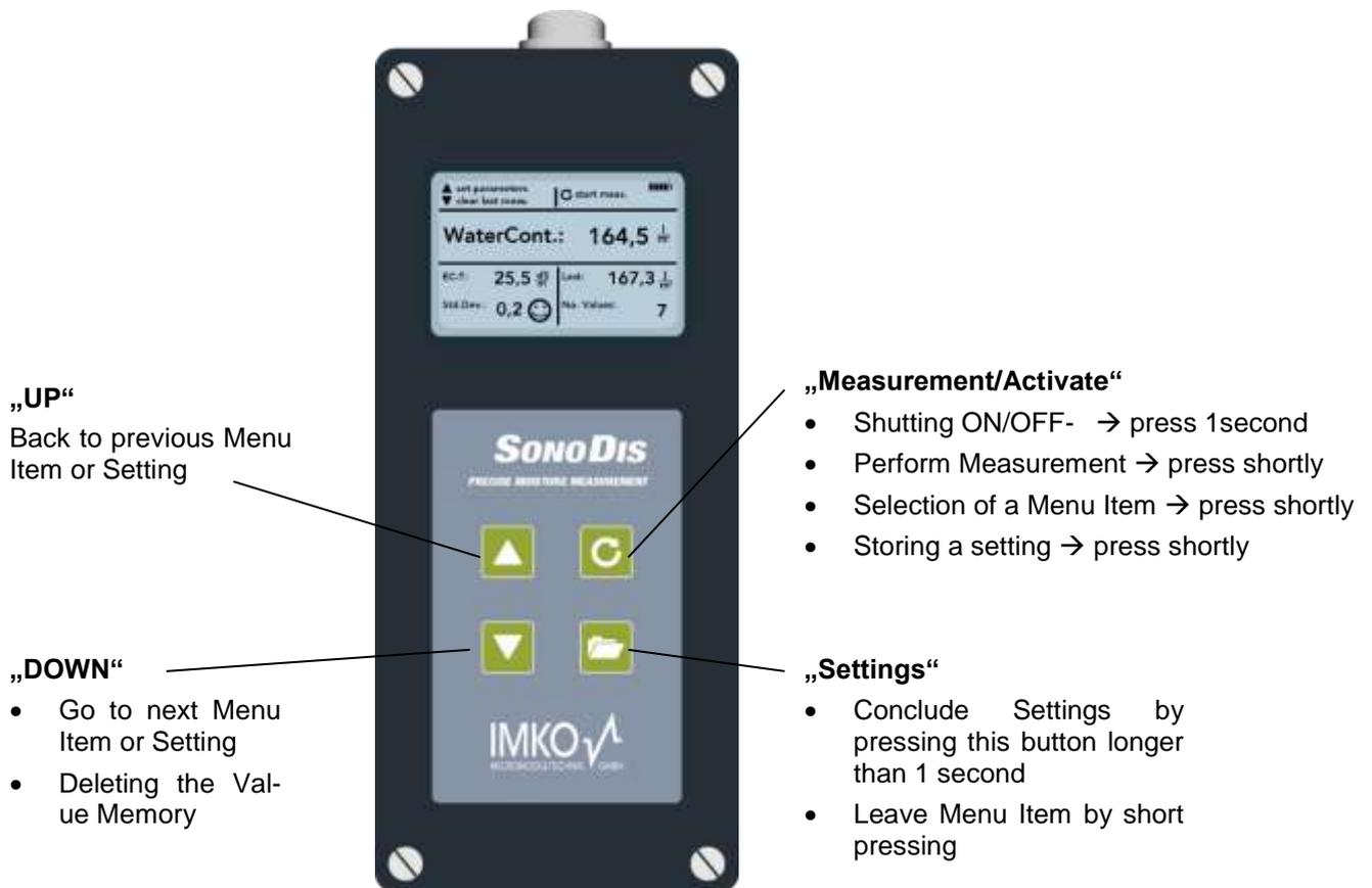
**Attention:** For measuring concrete, the standard calibration curve **“Cal. No.4”** is pre-selected inside the SONO-DIS. When switching on the SONO-DIS, the display shows the active calibration curve Cal.No.4. This pre-selection should be changed only if other materials as concrete like ceramic suspension, etc. should be measured.
