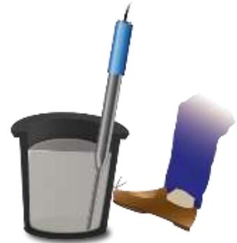
**Use a standard 10-12 liter plastic bucket. Do not use metal buckets or larger containers, due to correctly compaction!**
