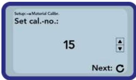
First you have to set the calibration curve to be changed (01 – 15) by pressing the buttons „Up“
