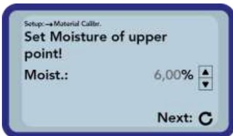
Next set the moisture of the higher moisture point by pressing the buttons „Up“
