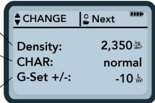
If you want to measure the complete water content (the total kiln drying water content) with SONO-WZ, the G-Set is to be entered with a plus value, with 1/3 of the core water!
