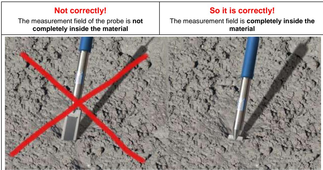
When inserting the probe several times at the same place, there is the danger of segregation effects at this place. By removing the probe out of the fresh concrete, the space will be filled with fine and liquid particles which could lead to higher measurement values.
