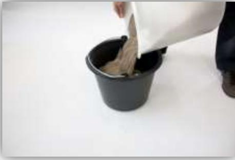
2. Compact the sand sample by lifting the bucket 5cm and letting it fall down vertically onto a solid base and repeat this procedure 5 times **(if there is still to see a compaction after 5-times repeat this procedure until there is no more compaction to see!)**
