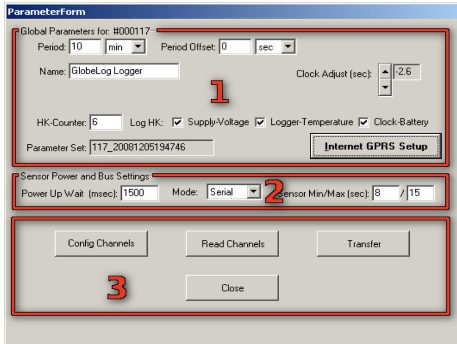
18. The parameter dialogue is divided into three areas: "Global Parameters" (1), "Sensor Power and Bus Settings" (2), and (3) in which the SM modules and channel configuration can be changed and transferred to the logger.
