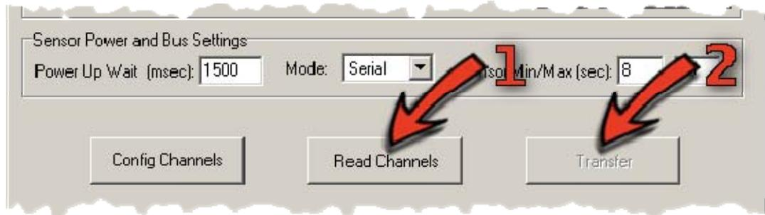
15. Here, first load the changed configuration file into the memory using the "Load Read Channels" button (1) and then transfer the new configuration to your globeLog using the "Transfer" button (2).
