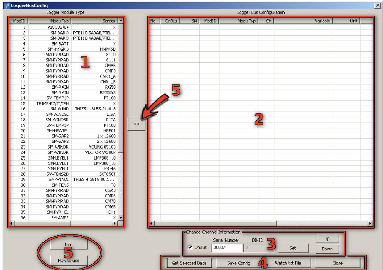
13. The window above is divided into five areas: "Logger Module Type" (1), "Logger Bus Configuration" (2), "Change Channel Information" (3), and "Help & Info" (4) and (5).
