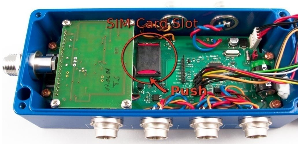
1. Open the SIM card slot by applying slight pressure to the lower end.
