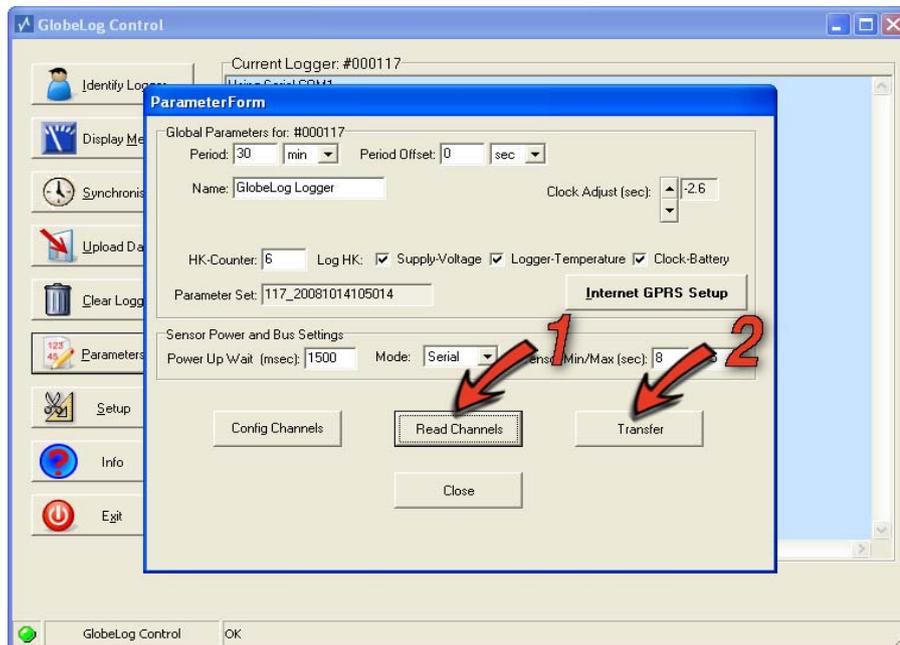
8. Next, load your configuration into the cache by clicking on the "Read Channels" button (1) and transfer them to the globeLog in a second step using the "Transfer" button (2). In doing so, the parameter dialogue closes and you find yourself back in the main window of the application.
