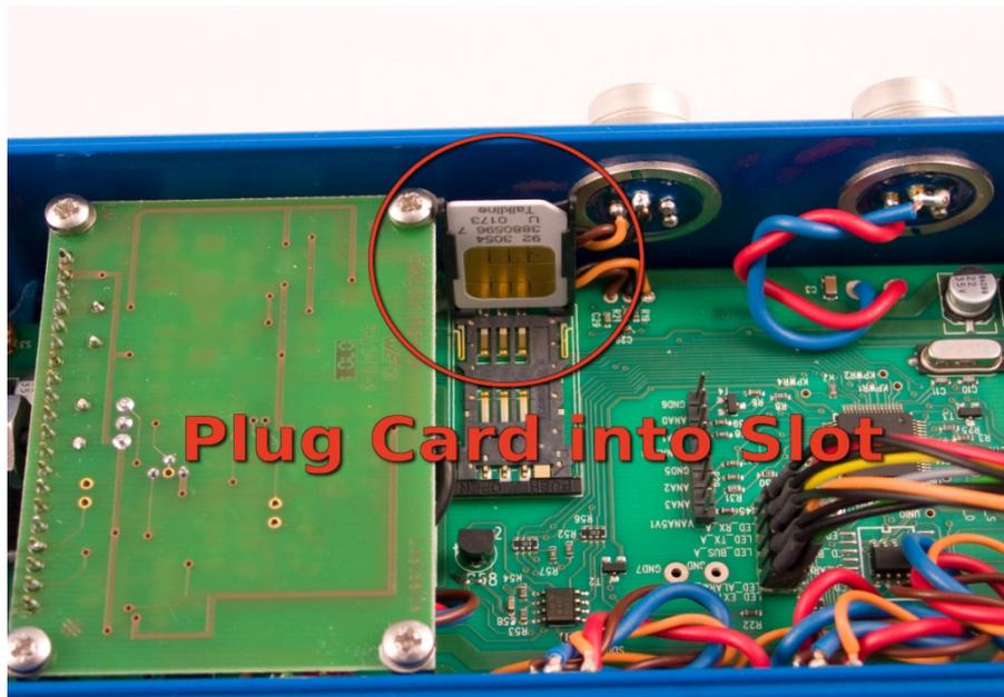
2. Insert the SIM card into the card slot.
