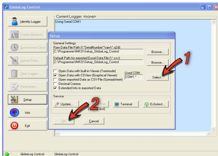
2. Here, select the computer's COM port you wish to use or the USB-RS232 adapter by clicking on the "Select" button (1). Close the setup dialogue using the "OK" button (2). If you have purchased a preconfigured globeLog System you can skip the following steps and continue
