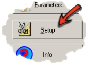
After starting globeLog Control, enter the setup dialogue by clicking on the "Setup" button. The following dialogue window appears:
