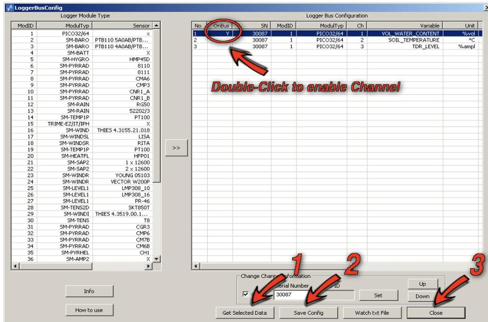
7. Now, by double-clicking, you can select the module channels to be measured. Then refresh your configuration using the "Get Selected Data" button (1), save your configuration with the "Save Config" button (2) and end this dialogue using the "Close" button (3). This returns you to the parameter dialogue.
