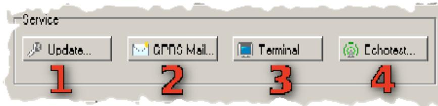
Button (1) opens a file-selection dialogue which enables you to load a new firmware into your globeLog. Button (2) sends an email via GPRS for test purposes to the email address specified in the GPRS setup. Button (3) opens a terminal that enables you to send direct commands to your globeLog. Button (4) starts a simple echo test and tests the logger's accessibility.
