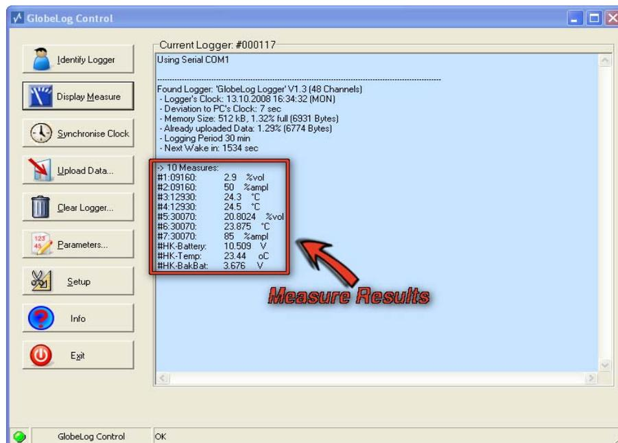
11. The readings are displayed in text form as shown above. This marks the conclusion of the basic configuration of the globeLog. For more detailed information about configuring the module channels, the measurement interval, and GPRS functionality, please read the following sections.
