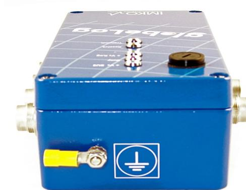
Surge-diverter connection (earthing!) Connect a Kreuzerder (grounding rod) or earthing strip here using a green/yellow earth wire (minimum diameter 6 mm<sup>2</sup>). Ensure that the connection is secured by means of stainless steel (V2A) screws, nuts etc.
