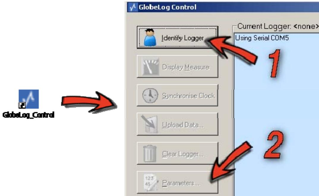
17. Identify your globeLog using the "Identify Logger" button (1) and then open the parameter dialogue using the "Parameters..." button (2). The following dialogue appears:
