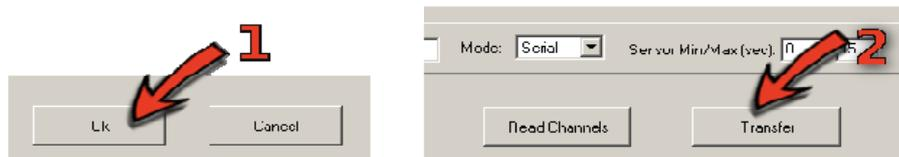
8. If you have changed settings in the GPRS dialogue, do not forget to **save** your changes using the “OK” button (1). When the GPRS dialogue has closed, you must still transfer the changed settings to your globeLog. To do so, click on the “Transfer” button (2) in the parameters dialogue.
