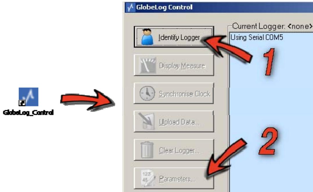
2. Identify your globeLog using the "Identify Logger" button (1) and then open the parameter dialogue using the "Parameters..." button (2). The following dialogue appears:
