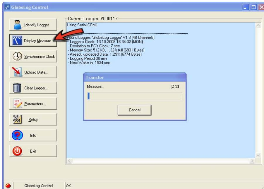
10. globeLog Control is now adequately configured for you to be able to perform a test measurement. To do so, click on the "Display Measure" "Display Readings" button. A dialogue opens that displays the progress of the measurement process. The measurement is complete as soon as this dialogue disappears.
