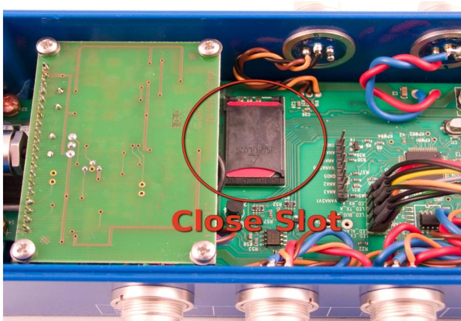
3. Close the card slot again by applying slight pressure.
