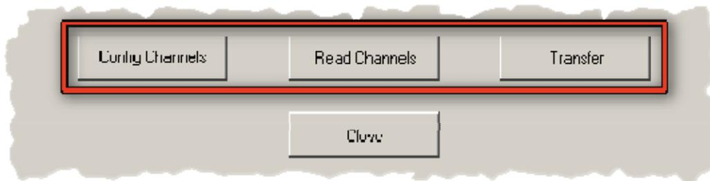
21. Area (3) contains the buttons to access the configuration of the SM module and sensor channels and to transfer the altered configuration to your globeLog. More details can be found in the section "Configuring the SM module and and sensor channels".
