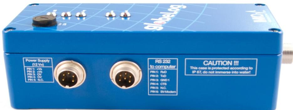
The other side of the casing has ports for the power supply (e.g.: for solar panels, batteries, or mains power) and the RS-232 port for communication with the aid of the globeLog Control Software (available at <http://www.imko.de>).
